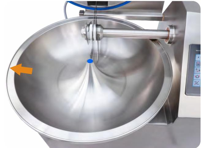
Solid **cast stainless steel bowl**. CNC precision machining, **with rim**.
