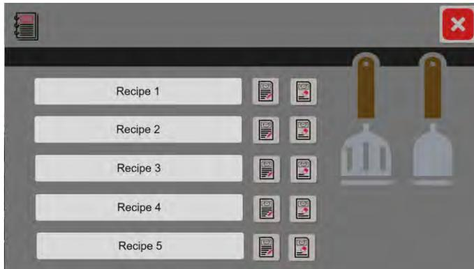
**Recipe function** allows standardization of recurring processes. Standard in TalsaControl 4.0
